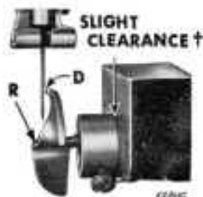
Fig. 11A. Locating Feed Eccentric and Looper
