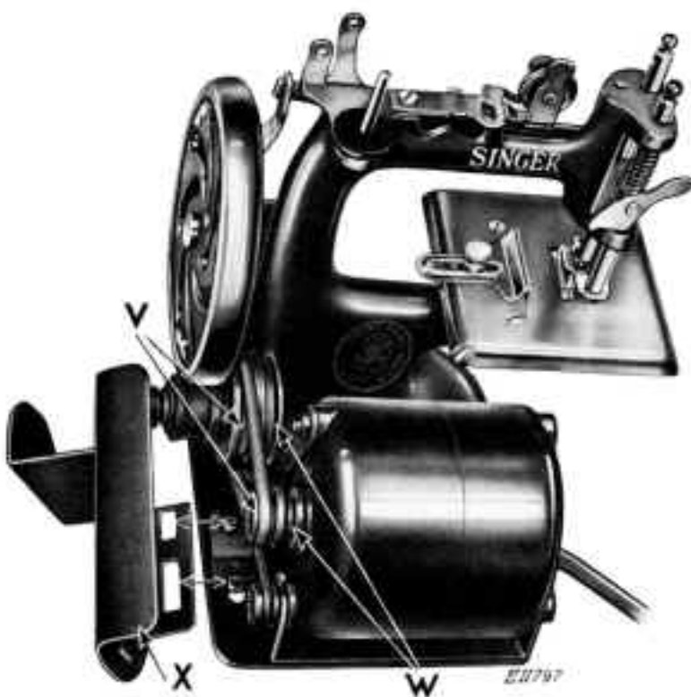
Fig. 19. Changing Speed of Machine 20-2
