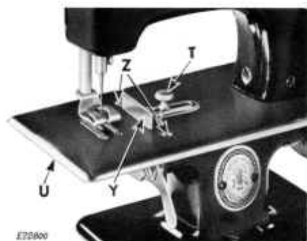
Fig. 12. Removing and Replacing Cloth Plate
